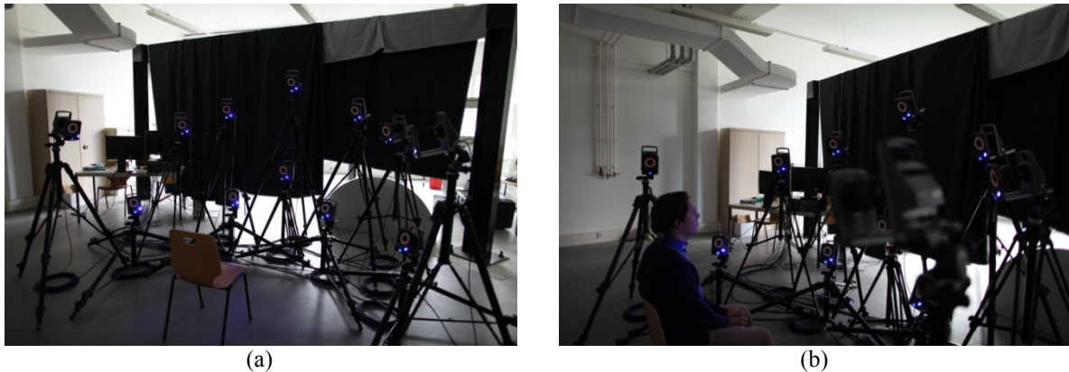
Fig. 1: Vicon system installation (a) 12 cameras positioned in a semi sphere (b) subject of the motion capture is placed just in front of the system.
